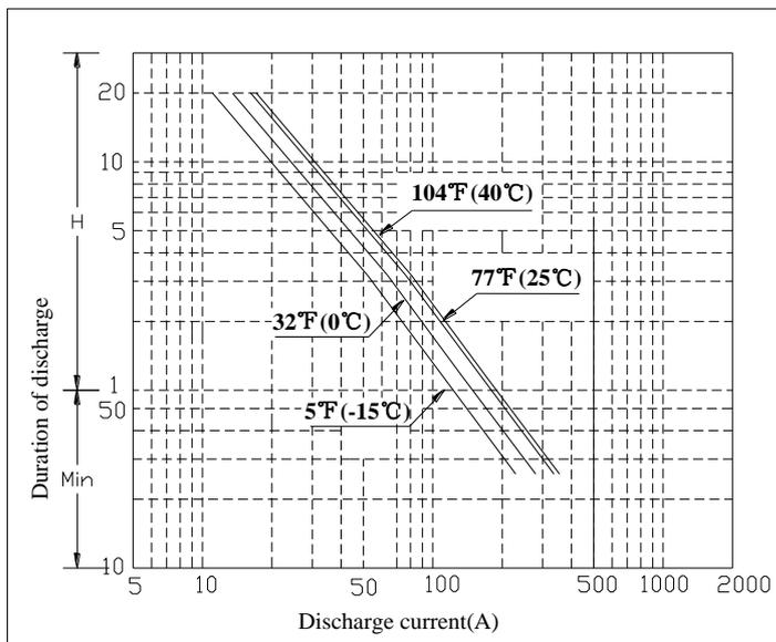
**Constant Current Discharge Rating Amperes @ 77 °F (25°C)**
